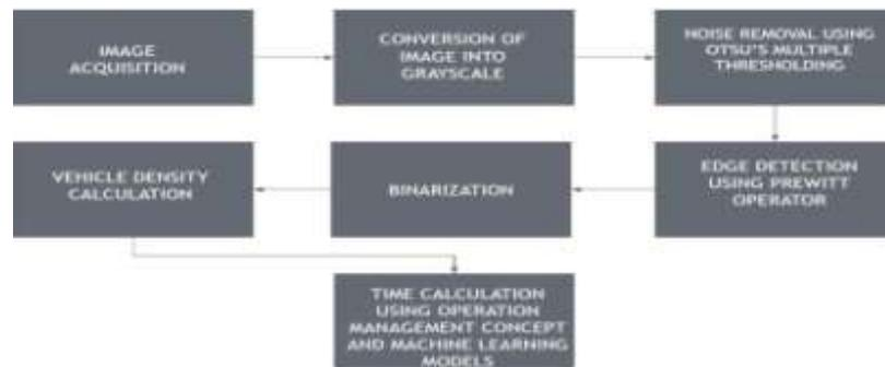
Fig. 1 Block Diagram of Traffic Congestion Management System
